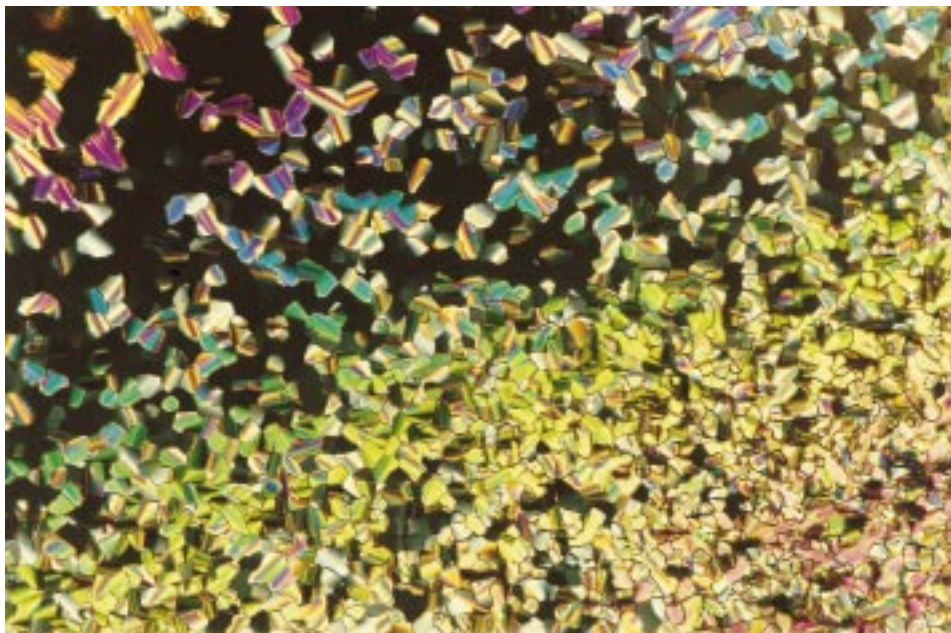
Fig. 2. Fan-shaped texture of the twin 9 . The photomicroscopic image of the mesophase was obtained with a polarizing microscope ( Olympus BX 50 equipped with a Linkam LTS 50 hot stage) at 13^\circ on cooling ( 0.2^\circ \text{ min}^{-1} ) from the isotropic liquid (crossed polarizers, magnification \times 200 ).
